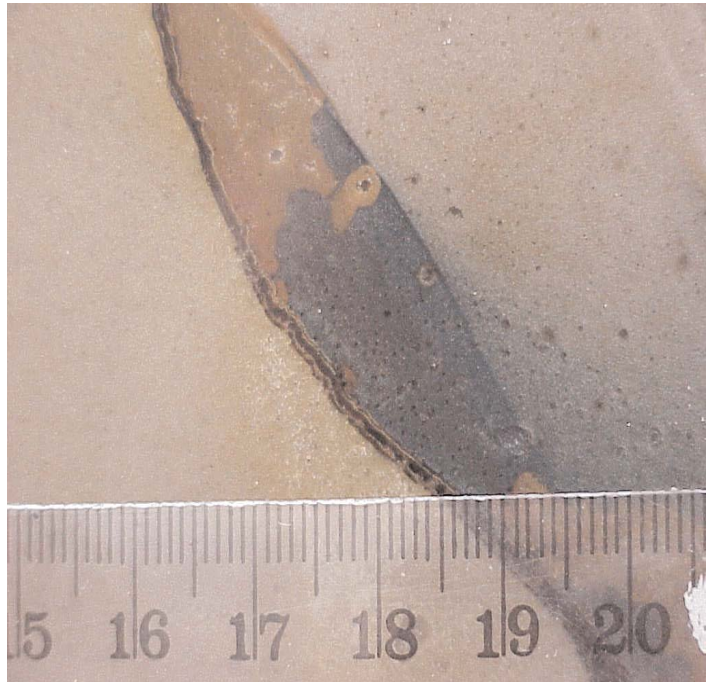
Figure 2: Sub-vertical, 1 cm thick Fe-rich band generated in water-saturated sands after 30 hours application of a 1.5 V potential difference between cast iron electrodes.
