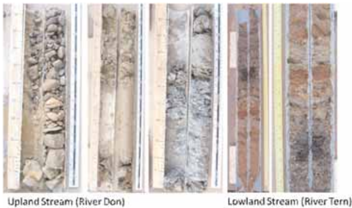
Figure 9. Riverbed cores from the River Don and River Tern (UK). Sampling cores is key to a better assessment of the physical and geochemical features of subsurface sediments which influence water exchange, transit times, microbiological activity and sorption potential for contaminants. (Pictures from T. Ibrahim (R. Don) and N. Riess (R. Tern)).
